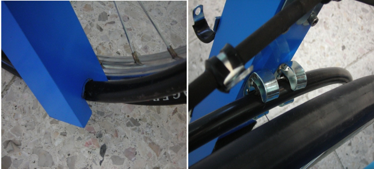
Figure 2: Left: The lower attachment point of RAE to the push rim of a wheelchair. RAE is able to pivot freely about this joint. Right: The upper attachment point of RAE to the push rim.
