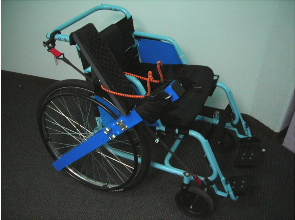
Figure 1: The Resonating Arm Exerciser (RAE) attached to a wheelchair in a right-handed configuration. A patient uses RAE by pushing rhythmically on the lever, rocking the chair at its resonant frequency.
