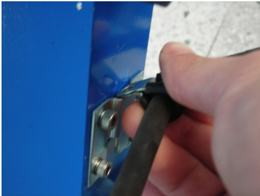
Figure 3: The attachment point between RAE and the elastic band. The tab on the elastic band fits securely into the slot on the side of RAE's main shaft and is held in place by the tension of the band. When RAE is not attached, the tab can easily slide to any point along the length of the elastic band where it remains during operation due to the friction of the rubber.
